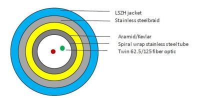
The ACP LaserTube cable is designed to be lightweight and flexible making it easy to handle and install and with a very fast thermal response time. In addition, the dual stainless steel and Kevlar protective layers provide excellent mechanical, tensile and pressure resistance (IP68 waterproof rating).
